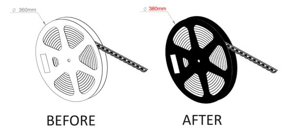
This change only affects to the diameter and color of the reel. Width and any other mechanical or electrical specification of the reel remain unchanged.
