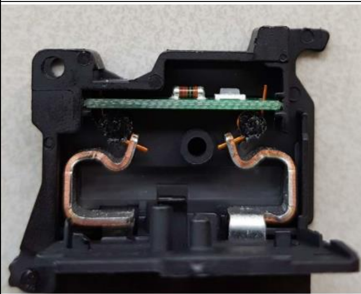
The addition of springs means that the HESI LED levers provide better contact quality.
