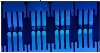
The lubricant is shown on the top row under the UV light source. The bottom strip is not lubricated.
