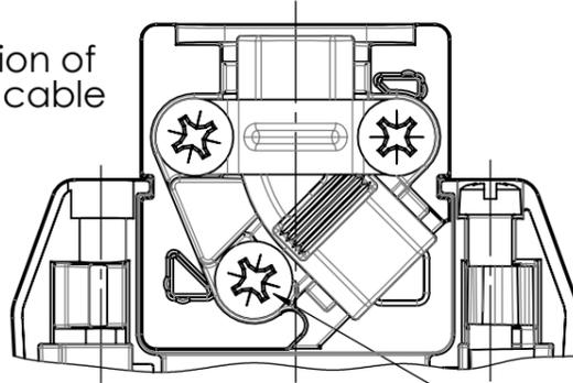
Installation of inclined cable outlet
