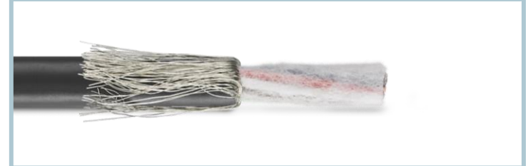
Fit the shield sleeve on the cable
